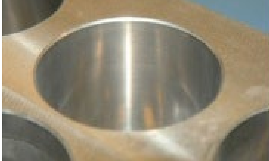
Good lubrication from Castrol Alusol produces a high-quality finish, 0.1 Ra (Roughness average) for precision components
